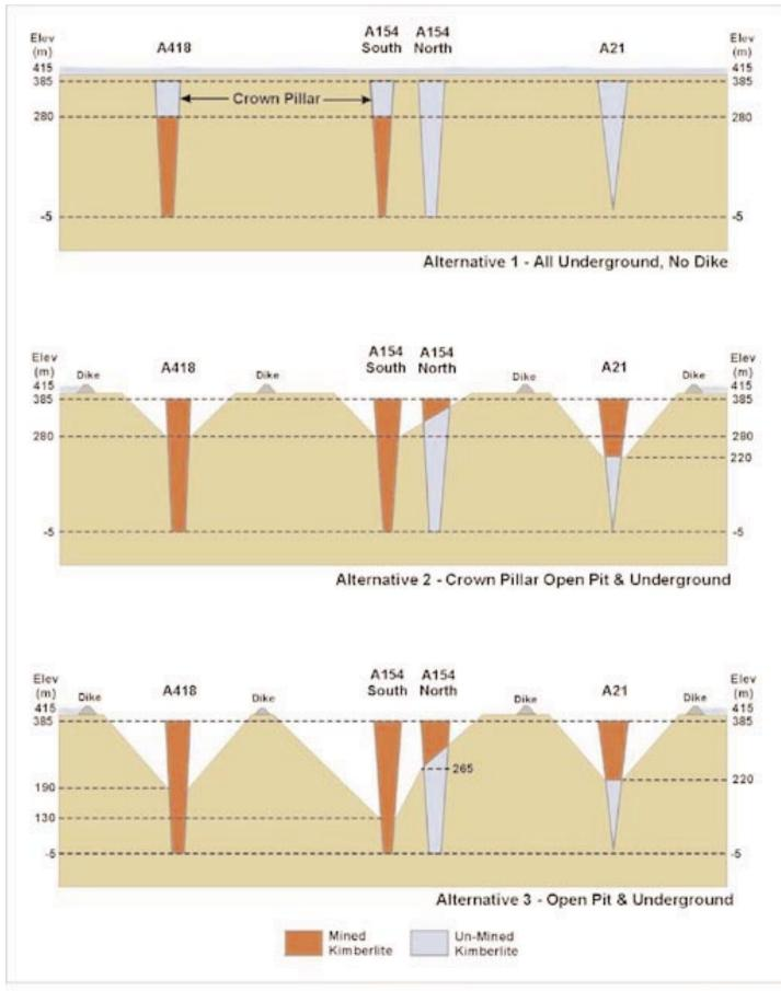
Figure 4-1 Schematic representation of three mining alternatives.
